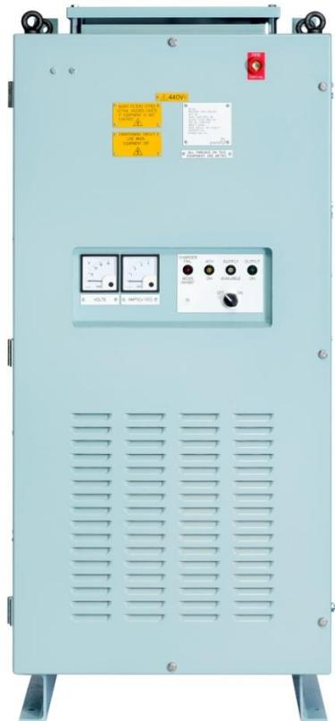
The Transformer Rectifier Unit 3RC15KG provides a high quality output of 27.4 volts dc with a continuous rating of 360A.
