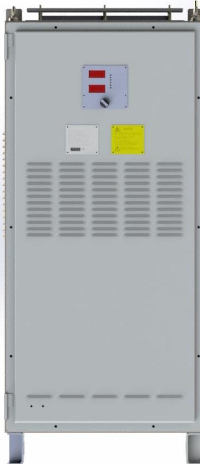
The 1CT3KB30A Static Frequency Converter (SFC) provides a high quality output of 115v 400hz 1 $\phi$  @ 3000VA from an input of 440v 50/60hz. The integral valve regulated lead acid battery will support the output for 30 minutes in the event of an input supply failure.
