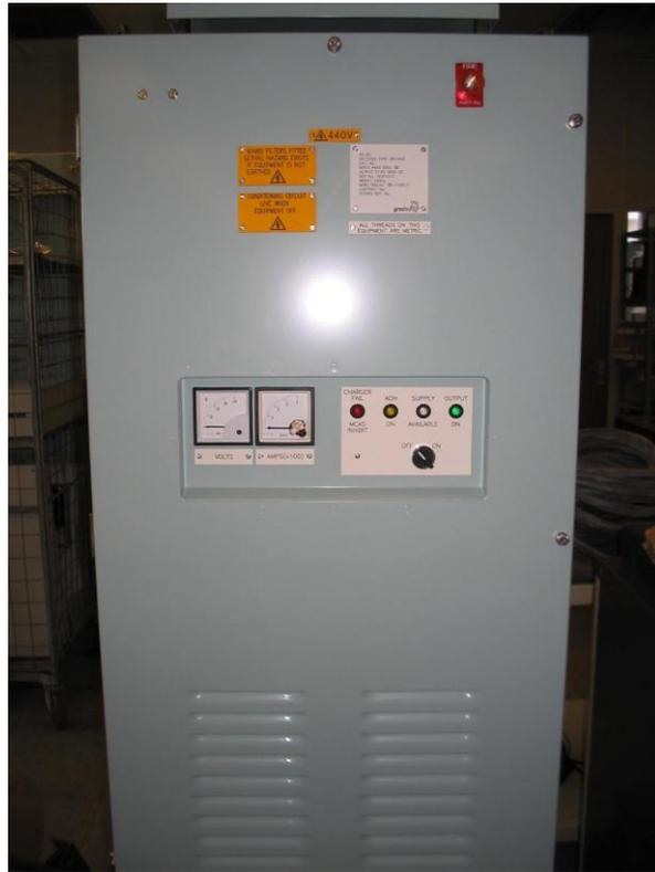
The Transformer Rectifier Unit 3RC10kF is intended for shipboard Helicopter Start applications. There are three basic modes of operation
