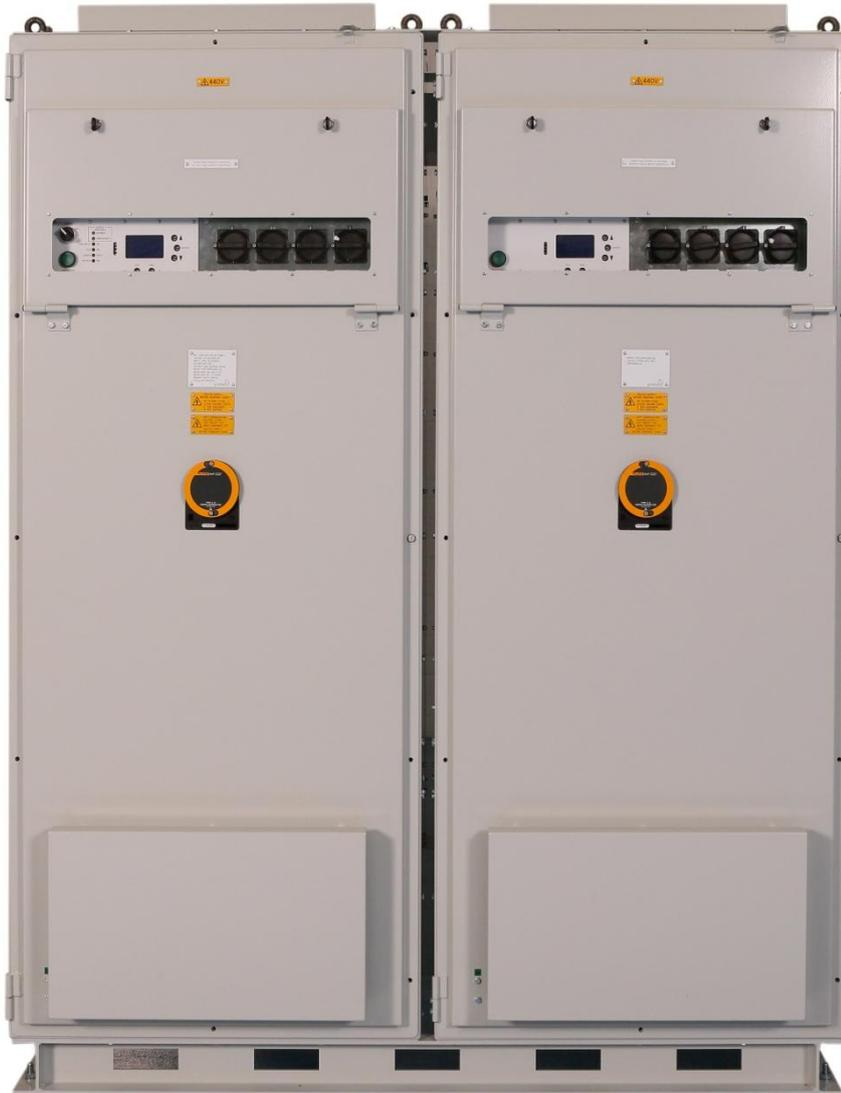
The 3RPQ30KA Uninterruptible Power Supply (UPS) supplies 230V, 60Hz three phase output to ships loads. The UPS consists of a transformer isolated rectifier, an inverter and static switch. An external battery cabinet is also required.
