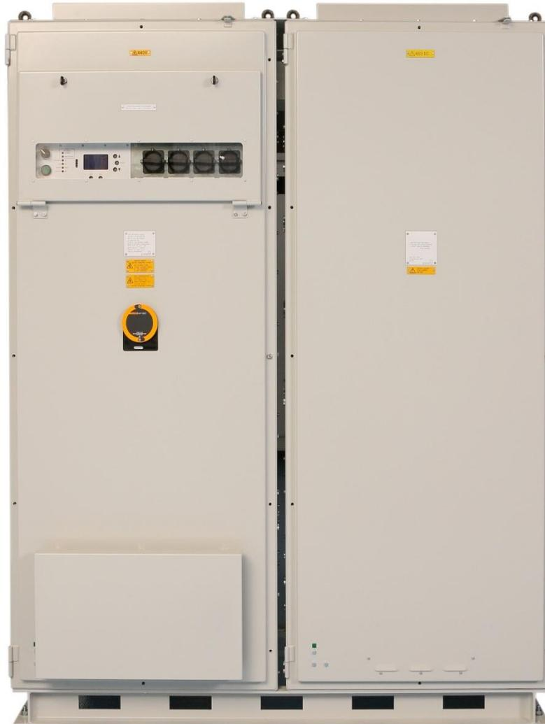
The 3RPQ15KB30A Uninterruptible Power Supply (UPS) supplies a battery supported, 115V, 60Hz three phase output to ships loads. The UPS consists of a transformer isolated rectifier, battery and an inverter.
