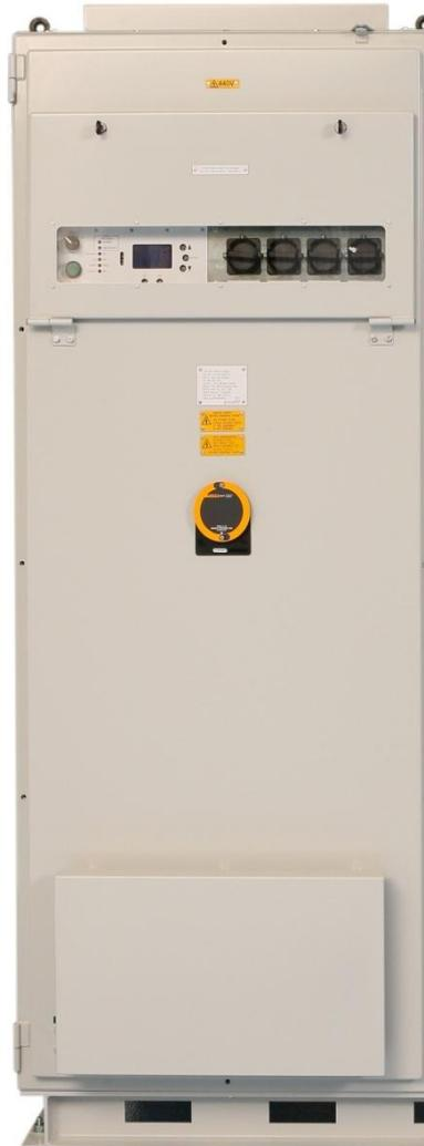
The 3RPQ15KB Uninterruptible Power Supply (UPS) supplies a battery supported ,230V, 60Hz three phase output to ships loads. The UPS consists of a transformer isolated rectifier, an inverter and a static switch. A separate battery cabinet is required.
