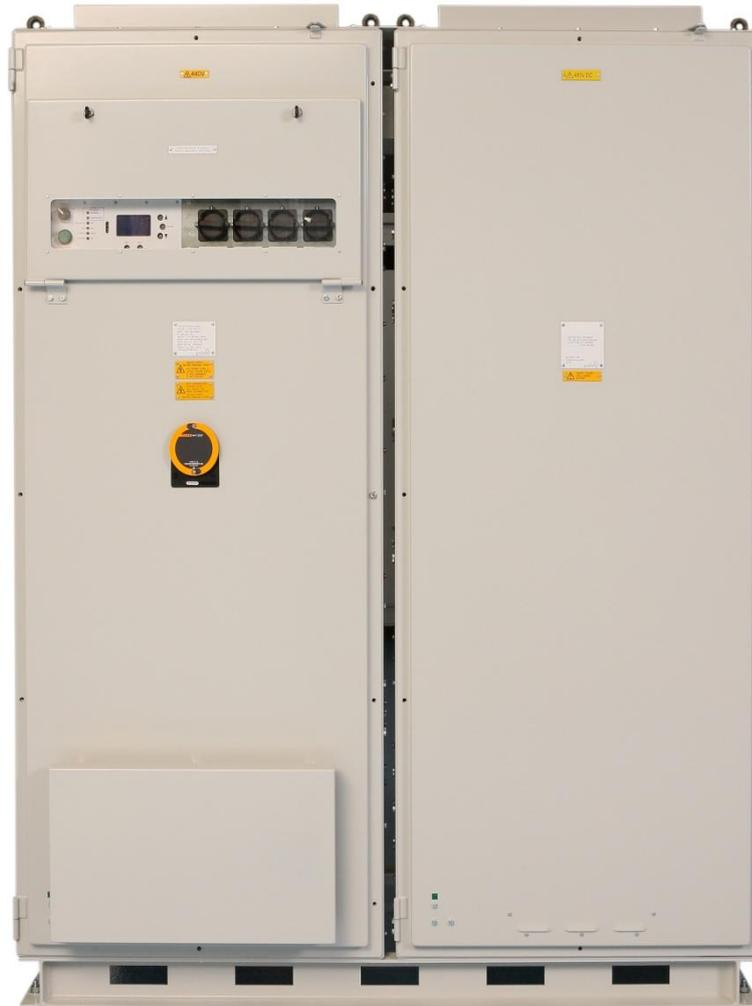
The 3RPQ Range of Uninterruptible Power Supplies (UPS) supply 60Hz three phase output to ships loads. The UPS consists of a transformer isolated rectifier, battery, an inverter and static switch. The batteries can be supplied either combined with the UPS or as stand alone cabinets
