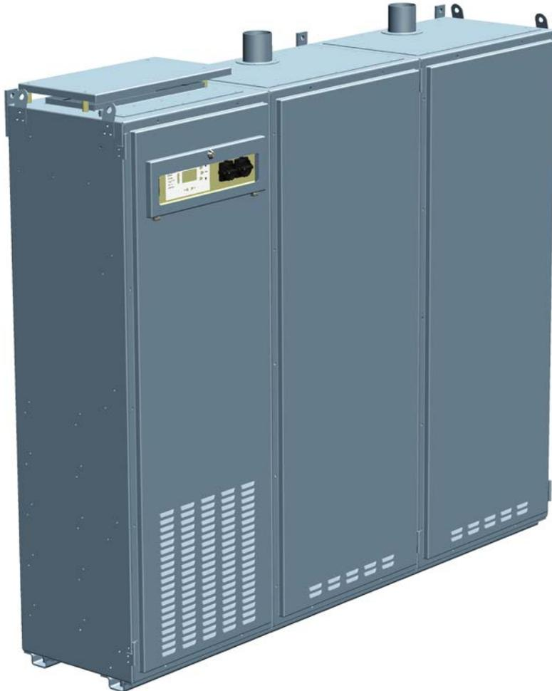
The 3RPQ Range of Uninterruptible Power Supplies (UPS) supply 60Hz three phase output to ships loads. The UPS consists of a transformer isolated rectifier, battery, an inverter and static switch. The batteries can be supplied nets either combined with the UPS or as stand alone cabinets
