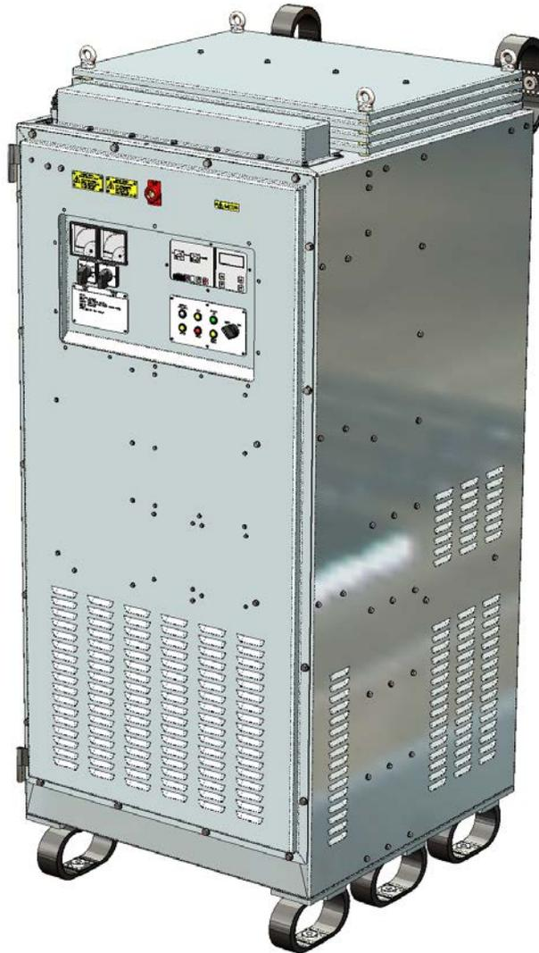
The 3CT40kB Static Frequency Converter (SFC) is designed to supply 3 phase(4wire) 200V, 400Hz to the aircraft loads with low distortion and high stability when connected to the ships' main 440 volt 3 phase 60Hz supply.
