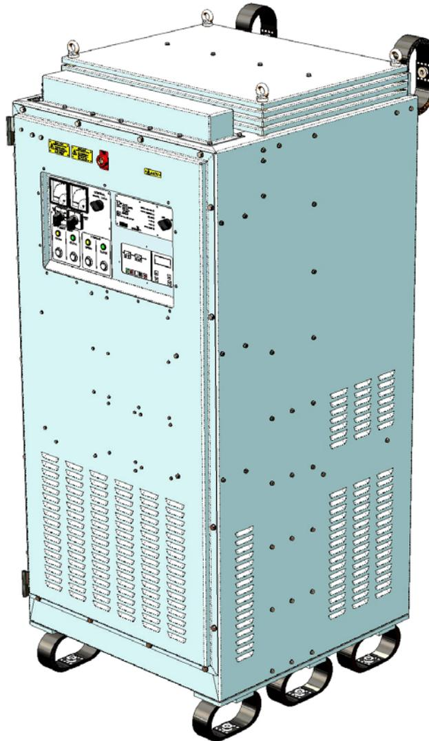
The 3CT40kA Static Frequency Converter (SFC) is designed to supply 3 phase(4wire) 200V, 400Hz to the aircraft loads with low distortion and high stability when connected to the ships' main 440 volt 3 phase 60Hz supply.
