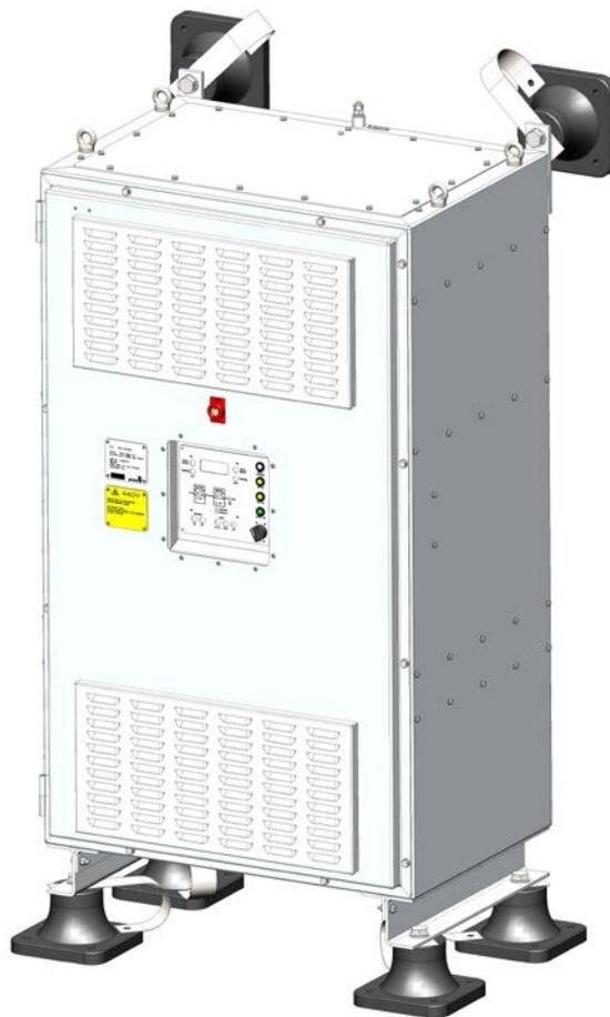
The 3CT Range of Static Frequency Converters (SFCs) are designed to supply 3 phase(4wire) 200V, 400Hz to aircraft loads with low distortion and high stability when connected to the ships' main 440 volt 3 phase 60Hz supply.
