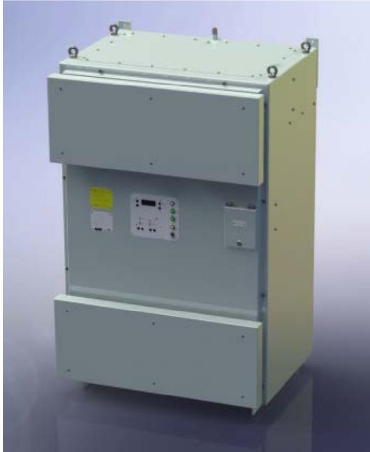
The 1RCQ10KA Uninterruptible Power Supply (UPS) supplies a battery supported, 115V, 60Hz single phase output to ships loads. The UPS consists of a rectifier and an inverter. A separate battery cabinet is required to house the associated battery.
