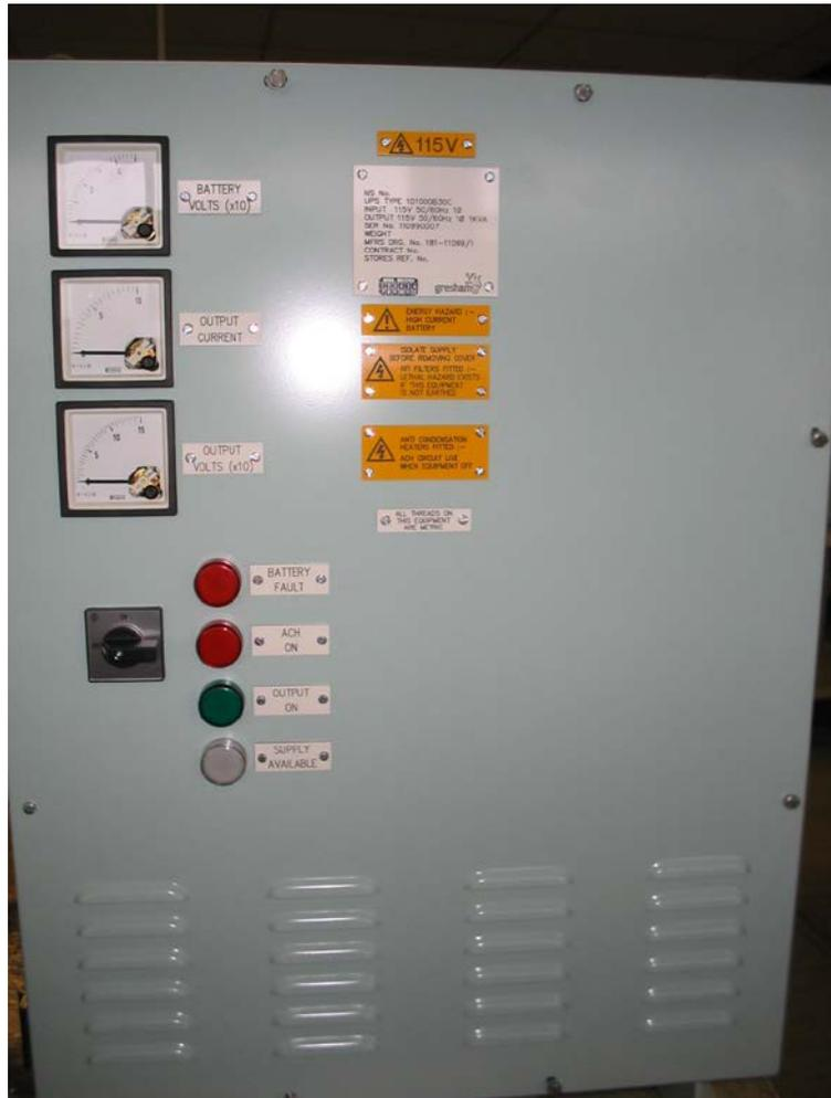
The 1D1000B30C Uninterruptible Power Supply (UPS) provides a high quality output of 115v 60hz 1 $\phi$  @ 1000VA from an input of 115v 50/60hz. The integral valve regulated lead acid battery will support the output for 30 minutes in the event of an input supply failure.
